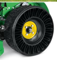
Optional X<sup>®</sup> TWEEL<sup>®</sup> TURF AIRLESS RADIAL TIRE by MICHELIN<sup>®</sup> All the qualities you want in a pneumatic tire, but none of the air – so flats
