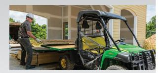
Removable composite side panels and tailgate lets you quickly convert the cargo box to flatbed operation for carrying a variety of bulky objects. 20 integrated tie-down points help you easily secure any load.
