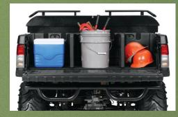
Easily repositioned Quick Clamp attachments like divider walls offer the ability to configure and reconfigure your cargo box in a few minutes with out tools.
