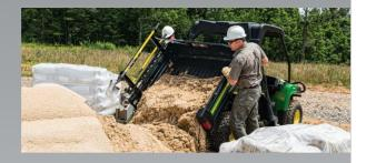
Easy-to-dump cargo box with standard gas-assist or optional automatic power lift. The standard gas-assist shock makes dumping effortless, while the optional power lift kit easily raises and lowers the bed with the press of a button.
