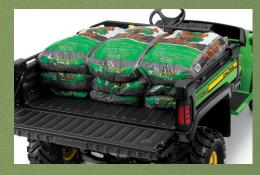
Cargo Box includes 16.4 cubic feet of capacity, pick-up style tailgate, 20 tie-down points, a gas-assist shock for easier lifting and dumping, and the ability to convert to a flat-had mode in minutes.
