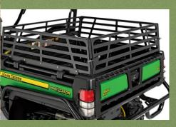
Optional Box Side Extensions increase the amount of light material you can haul such as clippings and mulch when compared to a base model cargo box. Tailgate pivots at the top for ease of unloading loose material.
